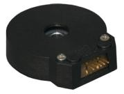
The ENC-A3I, is a high resolution single-ended encoder with an optional third index channel. This encoder requires a minimum shaft length of .445" and maximum shaft length of .575", and can be attached to shaft sizes ranging from .079" to 1" in diameter. The ENC-A3I provides digital feedback information for motion control applications that require position, speed and/or direction control.
