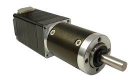
The 11YPG Series Gearmotor incorporates a high-torque stepper motor and an economic planetary gearbox to offer you an exceptional value. This compact package can deliver torque up to 833 oz-in. Gear ratios are available from 3.7 to 720. This gearmotor is ideal for applications that require high torque in a small package. The gearmotor can be customized to perfectly match your voltage, current, and maximum operating speed for maximum flexibility.
